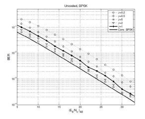
Fig. 3. BER of uncoded PNC with BPSK modulation for varying  $\rho$
